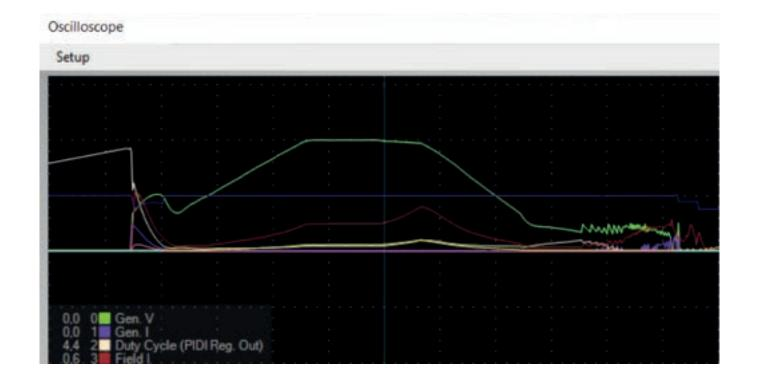
Above screenshot shows the Field Flashing and the Keep Alive functions effects during generator starting up and shutting down. Once the frequency drops below P.130 the AVR activates the keep alive function and works in order to maintain the excitation current to the P.250 keep alive setting (in this case 5%).
