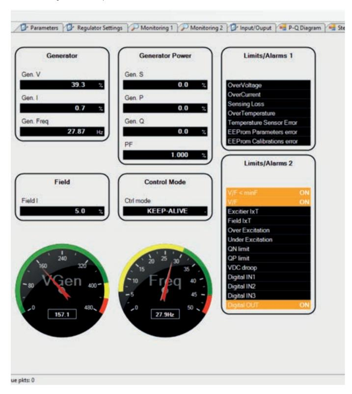
The reported limiters status shows that the V/Hz (underfrequency or underspeed) limiter is active.
