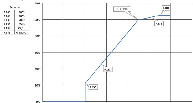
Note: The voltage corresponding at the minimum frequency (P.130) results from:
