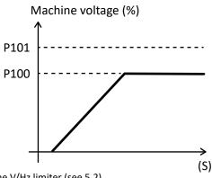
The voltage ramp is controlled also by the V/Hz limiter (see 5.2)
